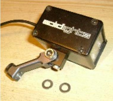
Assemble the adapter and light to your bracket using the M6 screw and nut. Since the walls of brackets vary in thickness, two washers are provided to fill any space if required. In the case shown they are not necessary.
