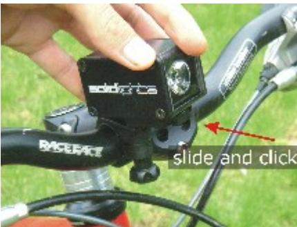
To attach the light to the bracket, slide it on to the bracket from the front. It will click into place.
