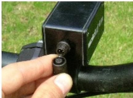
Attach the power cable from the battery to the light. The connector has a twist-lock action and will only fit one way round. Make sure the holes in the battery socket are lined up with the pins on the light. The connector should slide in quite easily – don't force it and risk bending the pins.
