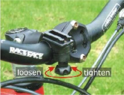
Your light is supplied with a quick-release handlebar mounting bracket. Attach the bracket to the handlebars in a convenient location using the thumbscrew.
