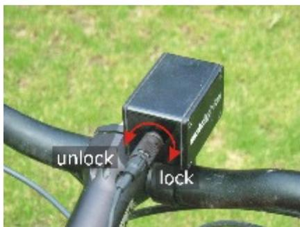
The barrel on the outside of the connector turns clockwise by just less than quarter of a turn to lock.
