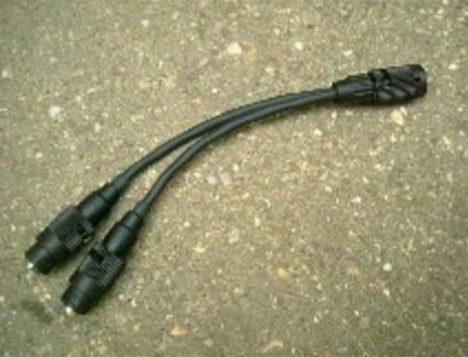
The battery doubler cable, part number 40012, is designed to allow two Solidlights Lithium Ion batteries to be connected to one Solidlights light unit, effectively doubling the run time. The cable contains special protection circuitry which ensures that charge is drawn evenly from the batteries and prevents damage to them.
