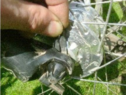
The Schmidt hub has two tags. Fit one terminal from the cable to each tag: it does not matter which way round they are connected.
