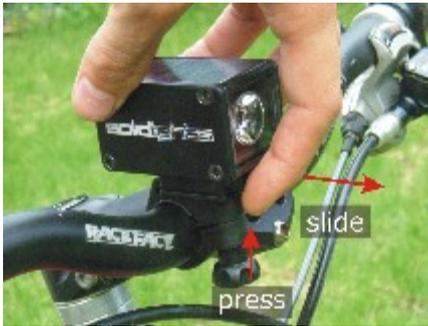
To remove the light from the bracket, hold the button underneath the front of the light and slide the whole light forwards. It should slide off the bracket easily.
