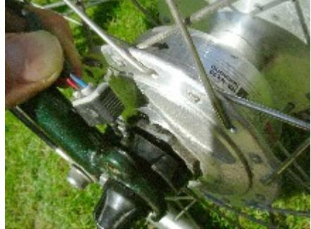
The Shimano hub has a single connector which will only fit one way round.
