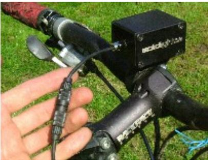
Attach the power cable from the battery to the flying lead on the light. The connector has a twist-lock action and will only fit one way round. Make sure the holes in the socket are lined up with the pins on the light. The connector should slide in quite easily – don't force it and risk bending the pins.
