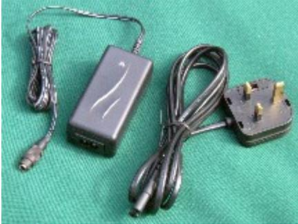
The Solidlights battery charger is a small, light unit using the latest switch-mode technology for maximum energy efficiency. It is compatible with mains power from 100 to 240 Volts, and so will work all over the world. It is supplied with a mains cable suitable for your country, but its socket will accept a standard 2-pin mains cable of the type normally used with radios and cassette players (IEC 320-C7, often known as 'figure-of-eight') so
