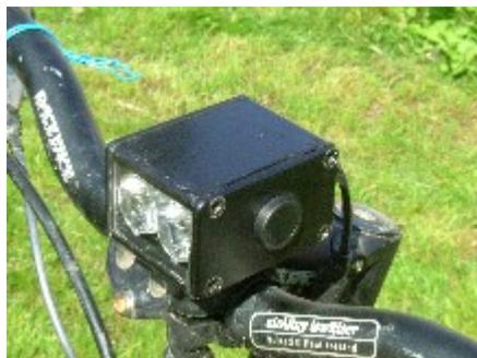
The light has just one control: the black button on the side. It's designed to be easy to operate even with gloved hands.
