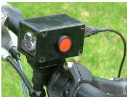
The light has just one control: the red button on the side. It's designed to avoid accidentally getting switched on and running your batteries down, and avoid accidentally getting switched off and plunging you into darkness on the trail.
